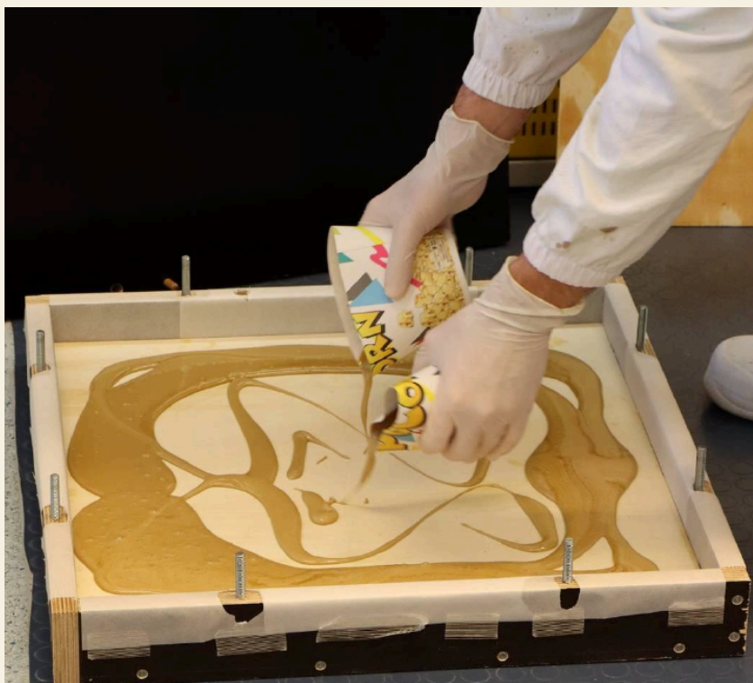
Figure 6: Pouring of the polyurethane foam mixture on top of the plywood
